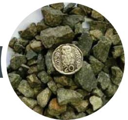
Note: WPB12 has a 35% void ratio and 100mm depth will store 300 litres/m<sup>3</sup>.
