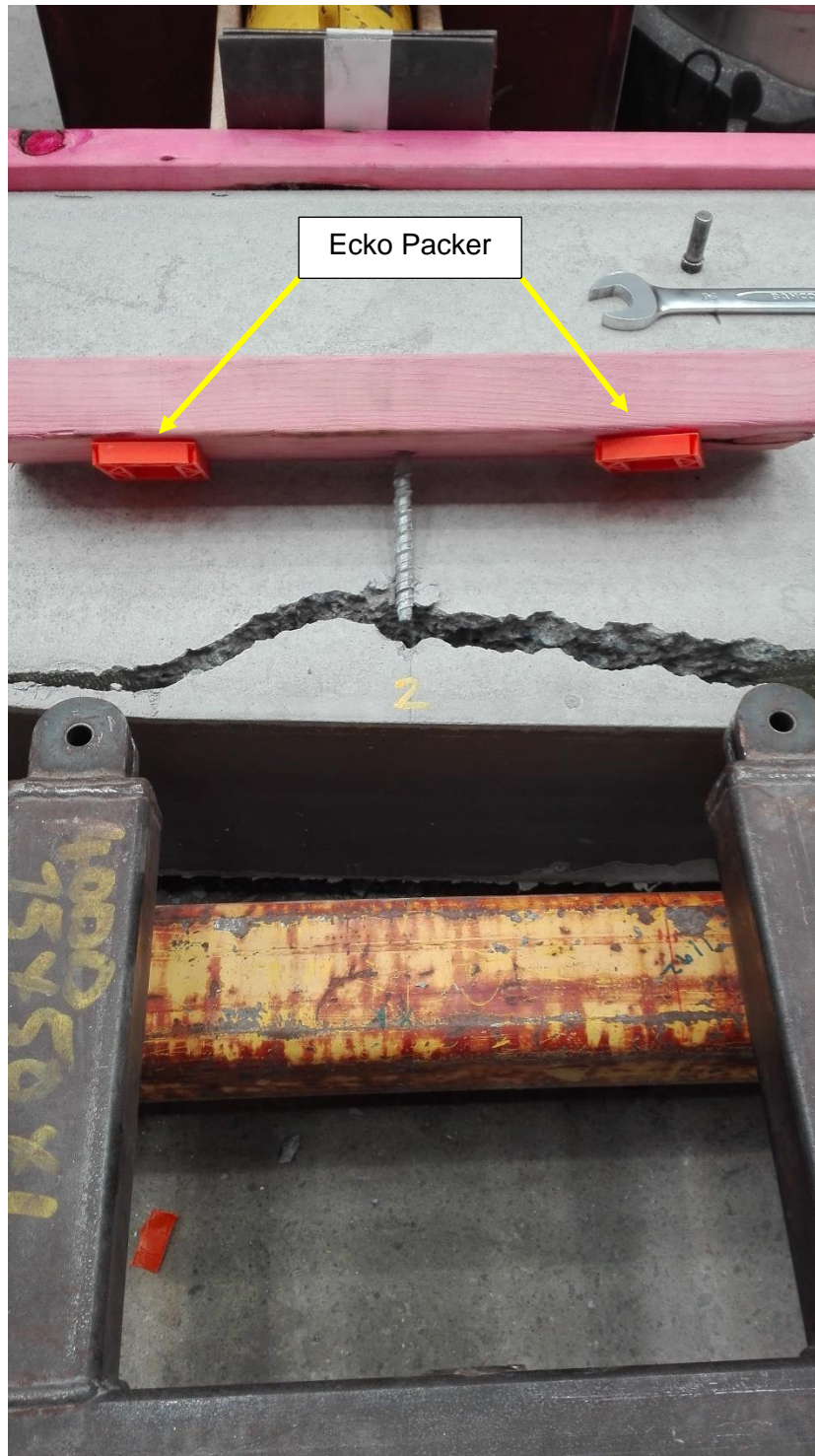
Figure 6 Concrete break out from Out of Plane testing
