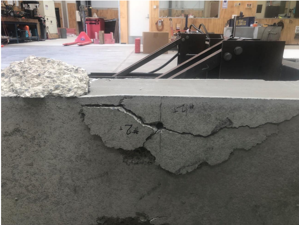
Figure 7. Failure by concrete edge breakout during tension testing.
